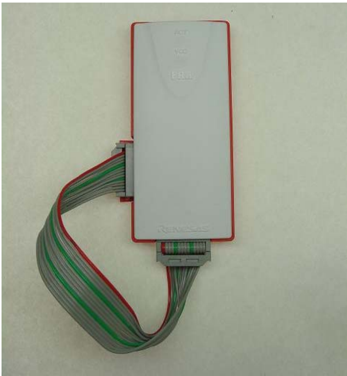
Figure E.1 Connecting the User System Interface Cable when Using the E8aSCP
